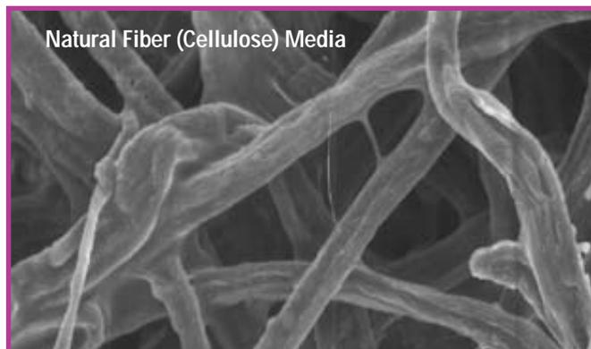
Media is, of course, the main factor influencing pressure drop; indeed, it causes pressure drop. That's why having a low-friction, high-flowing media is so important. See the differences in media in these close-up photos from our scanning electron microscope in which the media mat is magnified hundreds of times.
