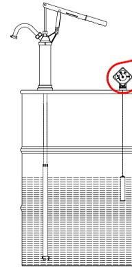
Fits the smaller 3/4" hole on drums, leaving the 2" hole free for installing pumps
